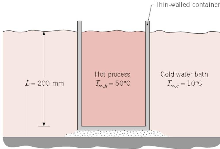
Note: Estimate the temperature of the wall as the average between the hot and cold fluid temperatures. Estimate the physical properties of the hot and cold films at 310K and 295K respectively (how does this compare to the exact average temperature for each film?).
