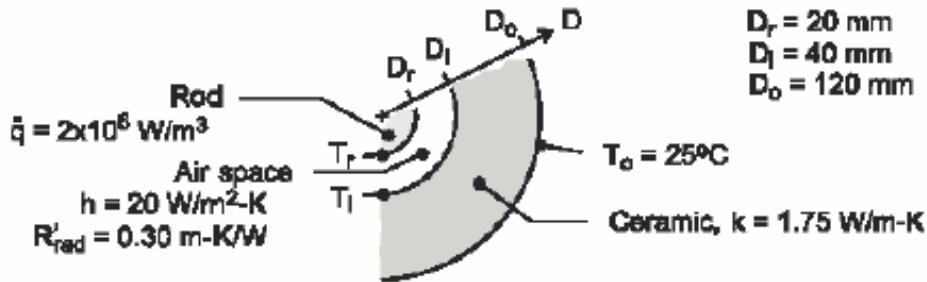
Assumptions: i) steady state, ii) 1D radial conduction, iii) free convection and radiation in the enclosure
