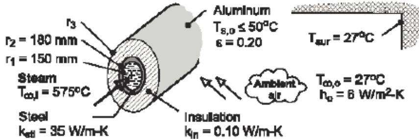
Assumptions: i) steady state, ii) 1D radial conduction, iii) negligible contact resistance at all interfaces, iv) negligible steam side convection resistance, v) negligible conduction resistance for aluminum sheet, vi) constant properties vii) large surroundings.
