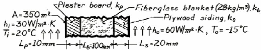
Assumptions: i) 1D conduction, ii) steady-state, iii) negligible contact resistance
