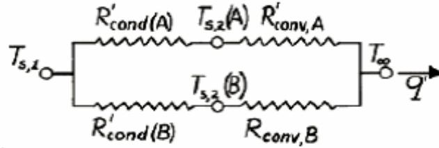
Because there is an infinite thermal resistance between the two insulating materials (i.e. no heat is exchanged between them), we can treat each insulating material as an independent heat transfer path. hence the two material are in parallel and the only two common values are the temperature of the inner wall  $T_{s,1}$  and the temperature of the surrounding air  $T_{\infty}$ .
