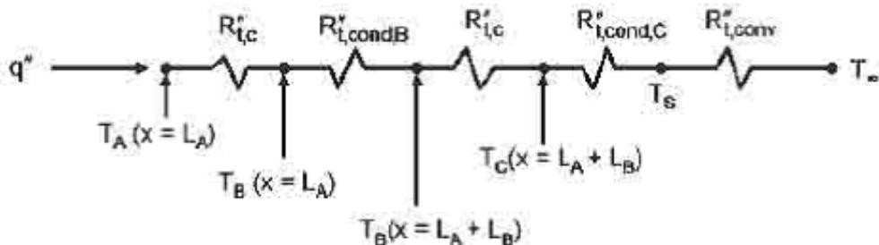
It is clear that  $T_A$  will be the maximum value for this part of the circuit. However, we know that heat is generated within the layer A and we thus expect a parabolic profile within such layer. Overall, the maximum temperature will thus occur at the adiabatic surface at  $x = 0$ .
