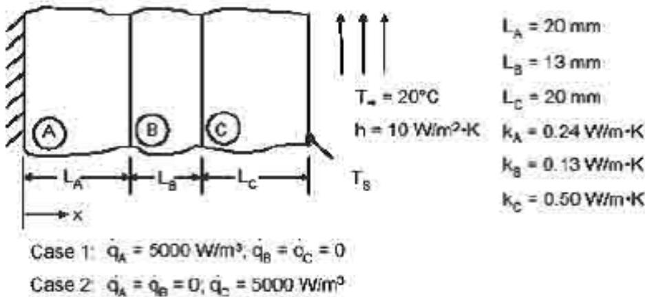
b) We first sketch the thermal circuit to help identify the important temperatures and heat transfer mechanisms (remember that the thermal circuit analogy is not valid in layers with heat sources, so in this case the layer A cannot be represented in the circuit).
