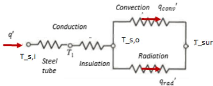
The thickness of the insulating layer must guarantee that, for an external surface temperature  $T_{s,o} = 50C$ , convection and radiation enable the dissipation of the necessary the heat transfer rate  $q'$ .
