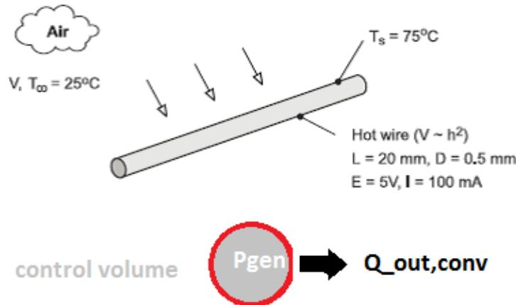
Assumptions: i) constant  $k$ ; ii) steady state; iii) negligible conduction and radiation b) The energy balance for the anemometer is
