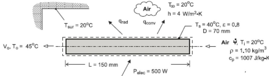
Assumptions: i) steady state; ii) constant air properties; iii) negligible potential and kinetic energy changes of air flow; iv) negligible work done by fan; v) negligible heat transfer from casing of dryer to ambient air.
