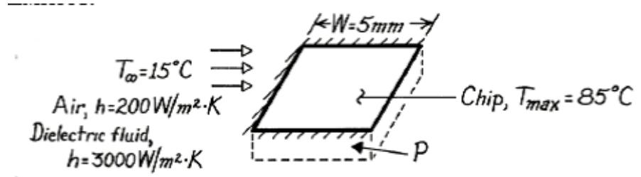
Assumptions: i) Steady-state; ii) isothermal chip; iii) negligible heat transfer through sides and bottom; iv) negligible radiative heat transfer.
