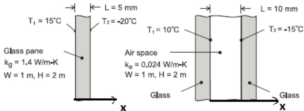
For the single pane window we express the conduction heat transfer rate as:
