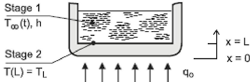
Assumptions: i) 1D conduction in the pan bottom; ii) uniform heat transfer from the stove to the bottom of the pan; iii) constant properties.
