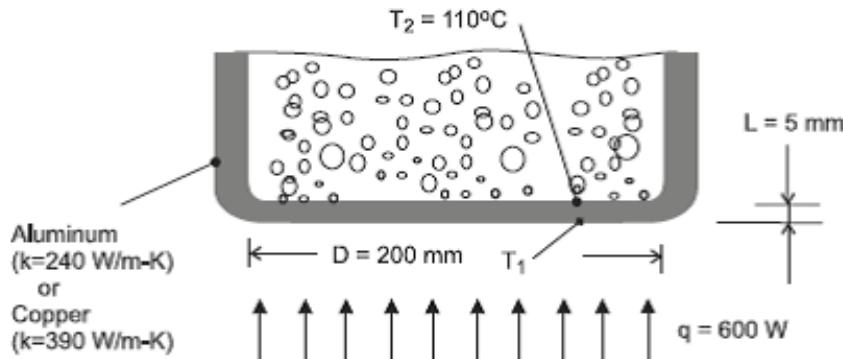
From the result of part c), using Fourier law we have that the heat transfer rate by conduction through the bottom of the pan is:
