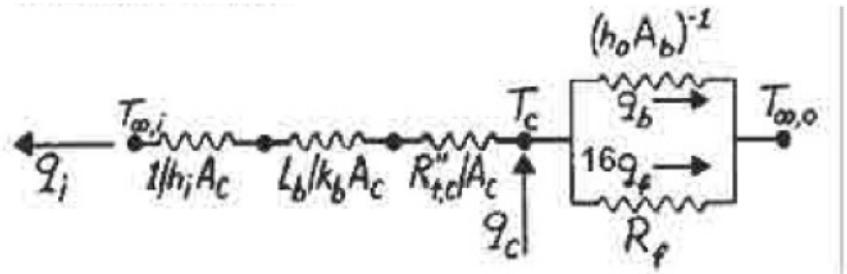
Note that we have indicated separate parallel paths for heat transfer through the fin and through the base of the fins. Also we have introduced the contact resistance between the chip and the fin.
