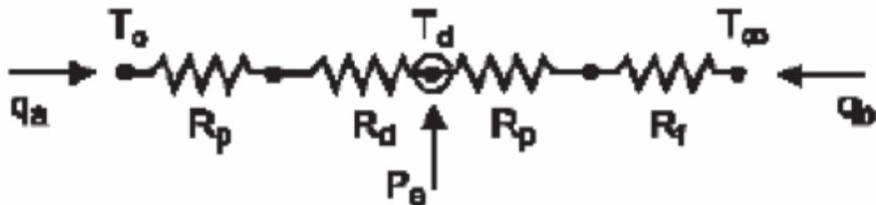
We want to first determine the thermal resistances. We know that we can neglect convection in the first part (pad + device + pad) and therefore conduction ALONG them is the only heat transfer mechanism. The thermal resistances are:
