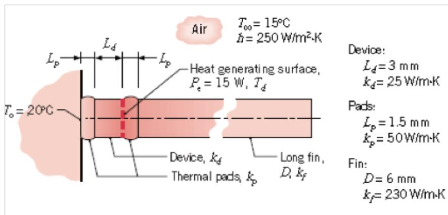
**Note:** considered the much shorter length of the thermal pads and electronic device compared to the fin, neglect the effect of convection along these parts.
