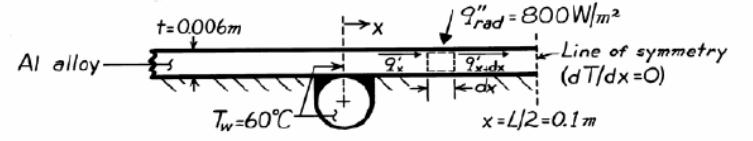
$$q'_x + q''_{rad}(dx) - q'_{x+dx} = 0, \quad \text{with } q'_{x+dx} = q'_x + \frac{dq'_x}{dx}dx \text{ and } q'_x = -kt \frac{dT}{dx}$$
