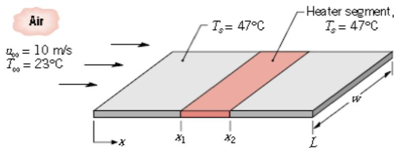
a) Estimate the electrical power that must be supplied to the designated heater segment to maintain the surface temperature at  $T_s = 47^{\circ}\text{C}$ .
