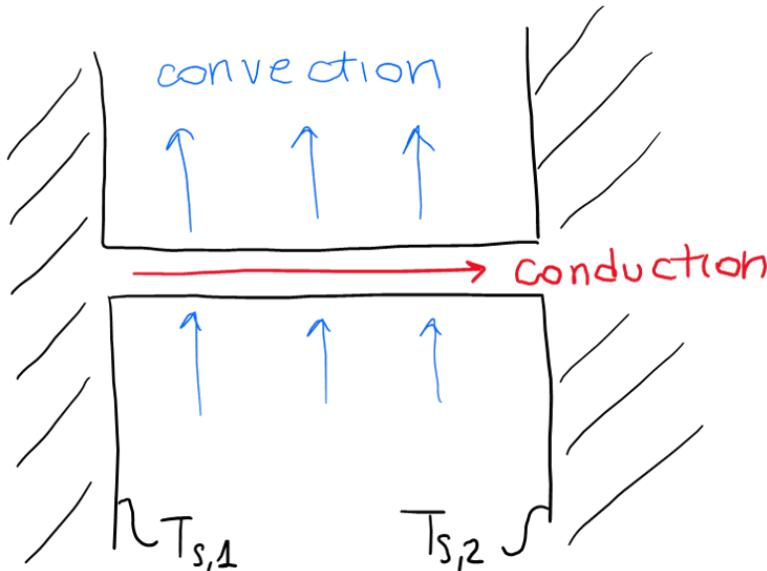
Each rod can be seen as a fin with uniform (circular) cross-section. Because the temperature is fixed on both surfaces, the temperature boundary condition must be applied at the tip.
