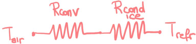
When the frost forms, the equivalent electrical circuit is composed of the frost conduction resistance and the convection resistance. We assume that the convection resistance is unchanged. The frost conduction resistance is equal to:
