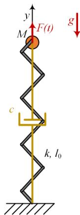
The system comprises mass  $M$  in a gravity field  $g$ . The mass  $M$  is attached to a spring ( $k$ ) and a linear damper ( $c$ ). The mass  $m$  is forced by  $F(t)$ . The governing dynamical equation of motion of the system is:
