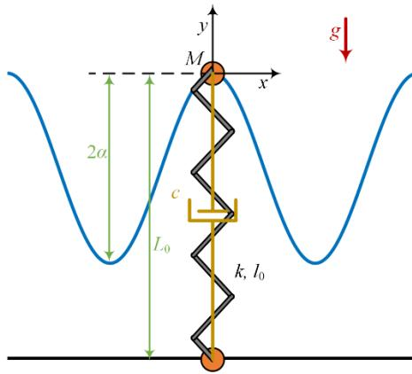
Instead of being driven by a harmonic force, consider that the system is constrained to move without friction on the blue sinusoidal rail, which is located at a distance  $L_0$  from the origin, as shown in the figure below. The attachment point between the spring, damper, and the ground is free to move along the black rail without friction. The blue rail is described by the function:
