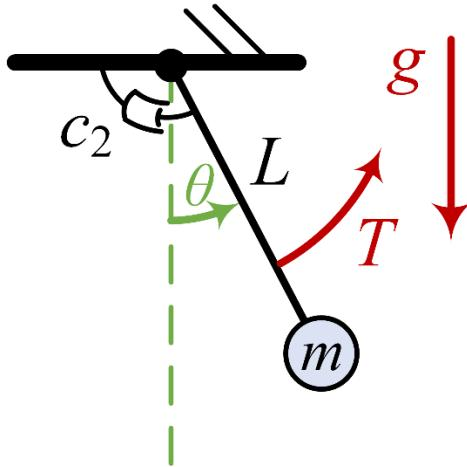
A weightless pendulum with length  $L$  and a point mass  $m$  at its end is connected to the wall with a joint, where the friction is modeled with an angular viscous damper,  $c_2$ . The input to the system is the torque  $T$ , and the output is the pendulum's angular position. The system is subjected to gravitation,  $g$ .
