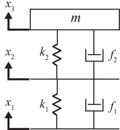
1. (10 points) Derive the transfer function  $G(s) = X_3(s)/X_1(s)$  of the system.
