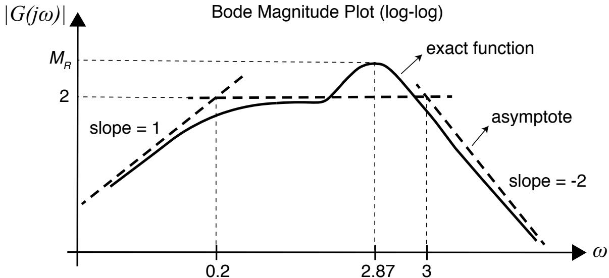
1. (7 points) Calculate the transfer function of the system given that there is no exponential term. What is the order of the system?
