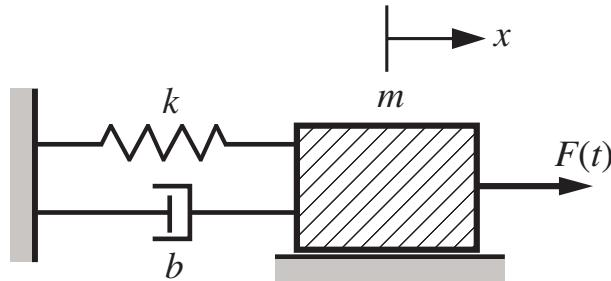
1. (10 points) Determine the numerical values of  $m$ ,  $k$ , and  $b$  so that when the input force is  $F(t) = 100\varepsilon(t)$  N
