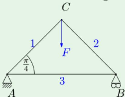
This triangular truss is made from steel with a Young's modulus of  $E = 200$  GPa and is loaded with a vertical force  $F = 20$  kN at node  $C$ .
