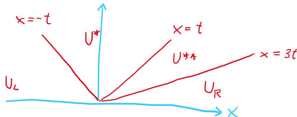
$$\begin{aligned} U_L &= \alpha_1 S_1 + \alpha_2 S_2 + \alpha_3 S_3 \\ U^* &= \alpha_1 S_1 + \alpha_2 S_2 + \beta_3 S_3 \\ U^{**} &= \alpha_1 S_1 + \beta_2 S_2 + \beta_3 S_3 \\ U_R &= \beta_1 S_1 + \beta_2 S_2 + \beta_3 S_3 \end{aligned}$$
