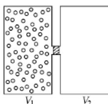
Gas is confined to a subvolume  $V_1$  in an insulated rigid container. The container has an adjoining subvolume  $V_2$ , initially evacuated, which can be connected to  $V_1$  by opening a valve ( $V_1 = V_2$ ). Suppose the valve is opened and the gas flows out of  $V_1$ , filling the entire volume,  $V_1 + V_2$ .
