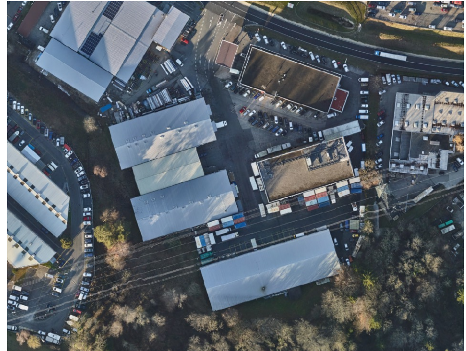
Ortho-rectified image (needs DEM) pixels correspond to \Delta x , \Delta y (m) on a projected surface
