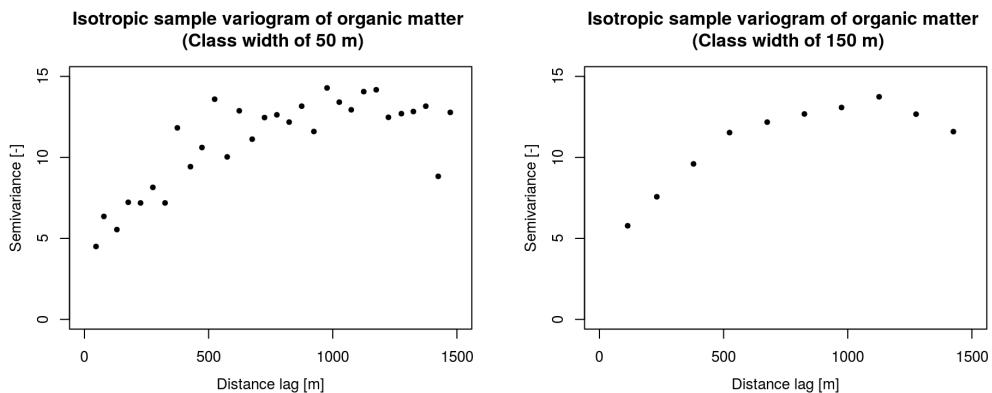
Smaller class widths allow to better estimate the spatial structure (especially at small scales) but the corresponding sample variograms are more noisy due to the larger sampling uncertainties (i.e., the semivariance estimates are less reliable because there are fewer
