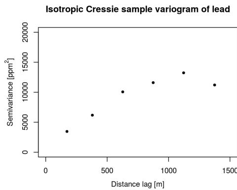
The values of the semivariances obtained using Cressie's estimator are smaller than the standard semivariance estimates. The estimated sill is about 12000 ppm<sup>2</sup> and the estimated nugget about 700 ppm<sup>2</sup> (5.8% of the sill). The range is practically identical (about 1000 m). The variogram obtained using Cressie's estimator is more representative because it is less influenced by the large concentrations values of lead (i.e., Cressie's estimator gives less weight to large values)
