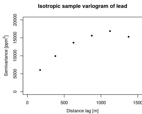
The estimated sill is 15500 ppm<sup>2</sup> and the nugget is about 2500 ppm<sup>2</sup> (16.1% of the sill). The range is about 950 m.
