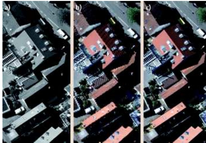
Figure 1.6: The concept of pan sharpening to increase the spatial resolution of color imagery. (a) High-resolution pan, (b) RGB low resolution, (c) RGB after pan sharpening, courtesy ifp-Stuttgart.
