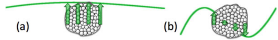
Fig. 2 Schematic showing (a) a particle small compared the wavelength (traced out by the green line) in which the electric field (green vectors) is uniform throughout the particle, and (b) a particle large compared to the wavelength in which the electric field is nonuniform throughout the particle. In (a), the induced dipoles oscillate in phase with one another. In (b), the induced dipoles oscillate out of phase with one another
