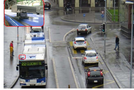
Fig. 3. One of our sensor nodes anchored to the roof of a Lausanne bus. The gas sampling system used in this paper is a sub-module of this real-world platform.
