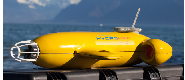
Fig. 1: The Vertex AUV with its sensor suite in the front, protected by a white cage. The AUV is about 70 cm long, weighs 7 kg, and can be carried and deployed easily by one person.
