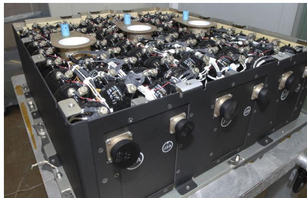
Nickel-Hydrogen batteries for Hubble
