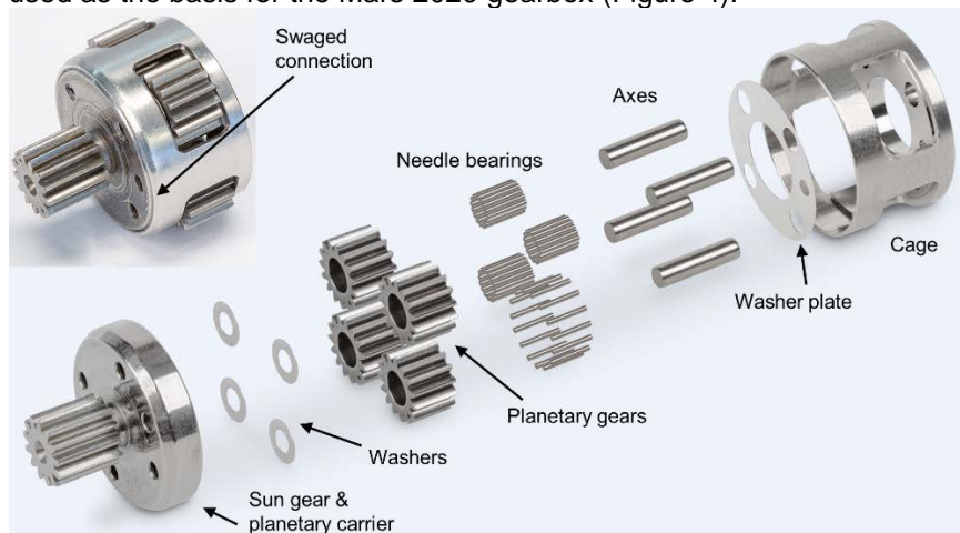
Figure 4. Exploded view of M20 planetary gearbox stage
