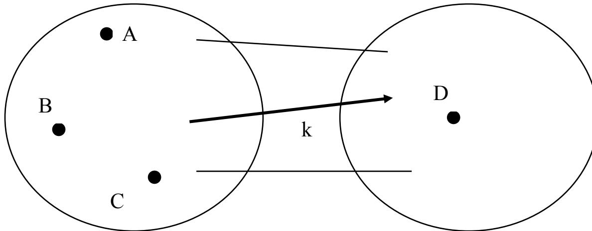
$$q_{AD} = 900 \text{ MW}, \text{PTDF}_{AD}^k = 0.1; \quad q_{BD} = 300 \text{ MW}, \text{PTDF}_{BD}^k = 0.3, \quad q_{DC} = 100 \text{ MW}, \text{PTDF}_{DC}^k = -0.2$$
