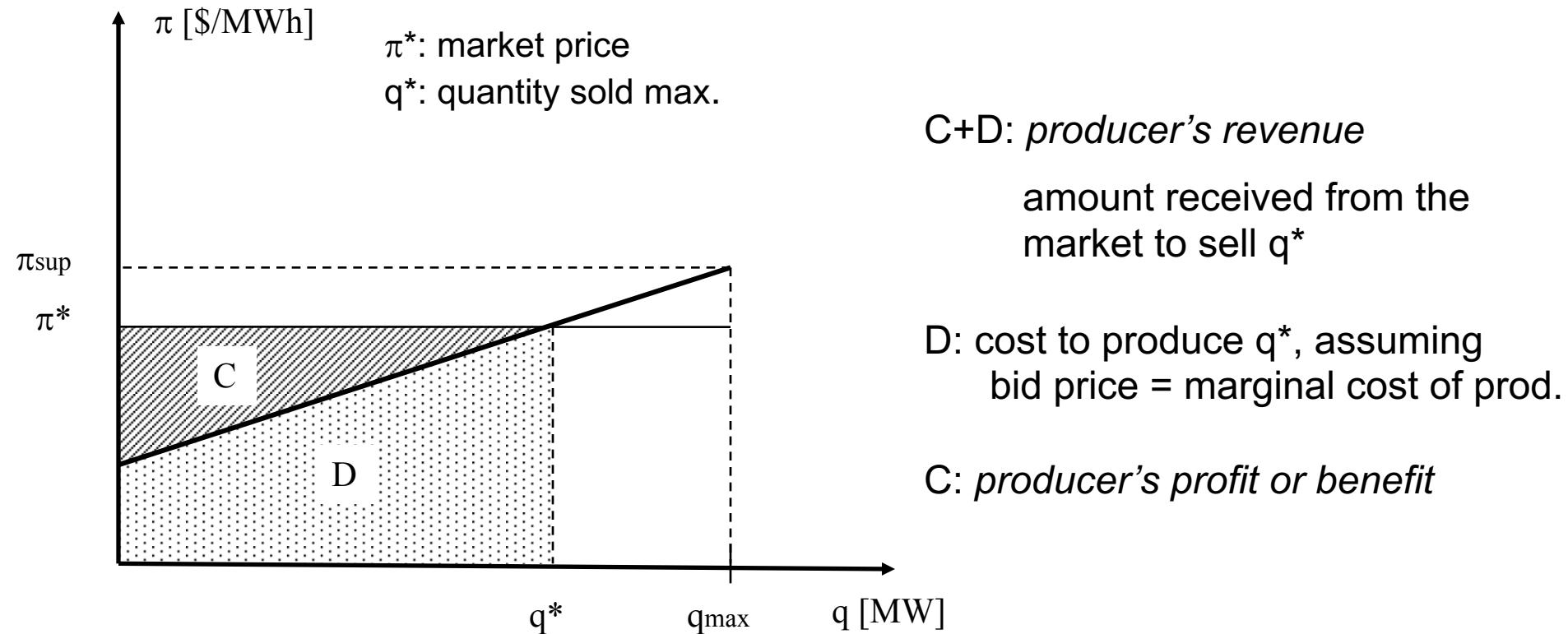
D corresponds to the *production cost function* or *curve*  $C(q)$  (\$/h or \$) if it includes the constant *no load* and the *startup* costs
