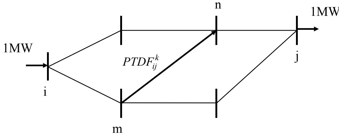
$PTDF_{ij}^k$  is defined as the fraction of MW flowing in line k (or m-n) resulting from 1 MW injected in node i and consumed in node j
