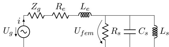
— If we introduce the equivalent electric impedance  $R_s = \frac{(B\ell)^2}{R_{ms}}$  :
