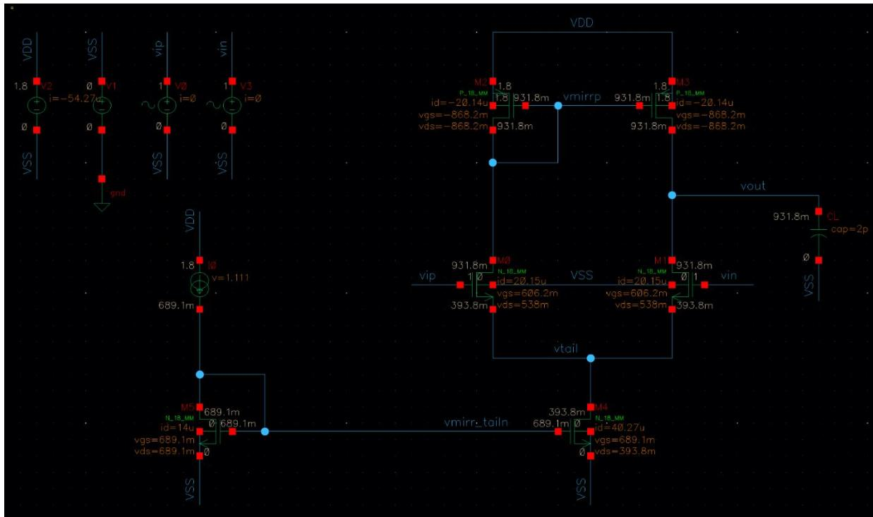
Click **Results>Print>DC Operating point**, then click on the transistor M0. In this list, you will find the small signal parameters that are derived from the transistor model and the bias point. Check for the different parameters that we designed for, namely,  $r_o$ ,  $g_m$ , etc. We note that the small signal parameters are reasonably close to the desired design value.
