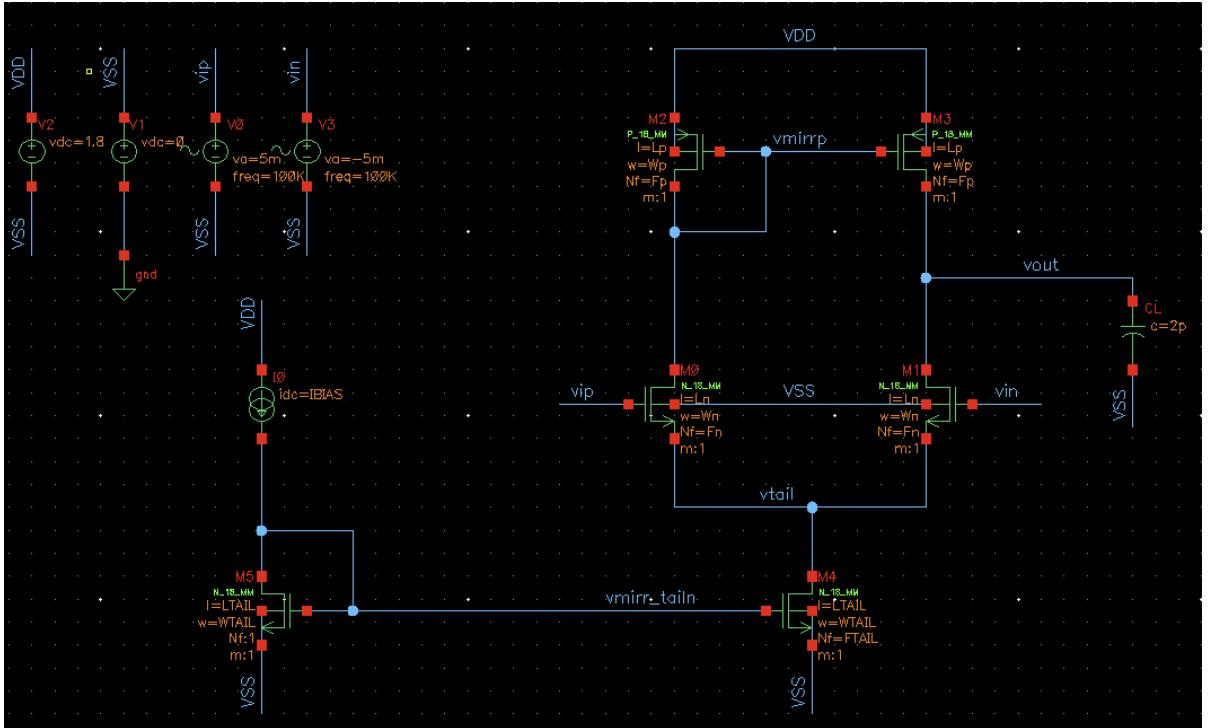
For the circuit, we know that the voltage gain  $A_v = g_{mn} \cdot (r_{on} || r_{op})$
