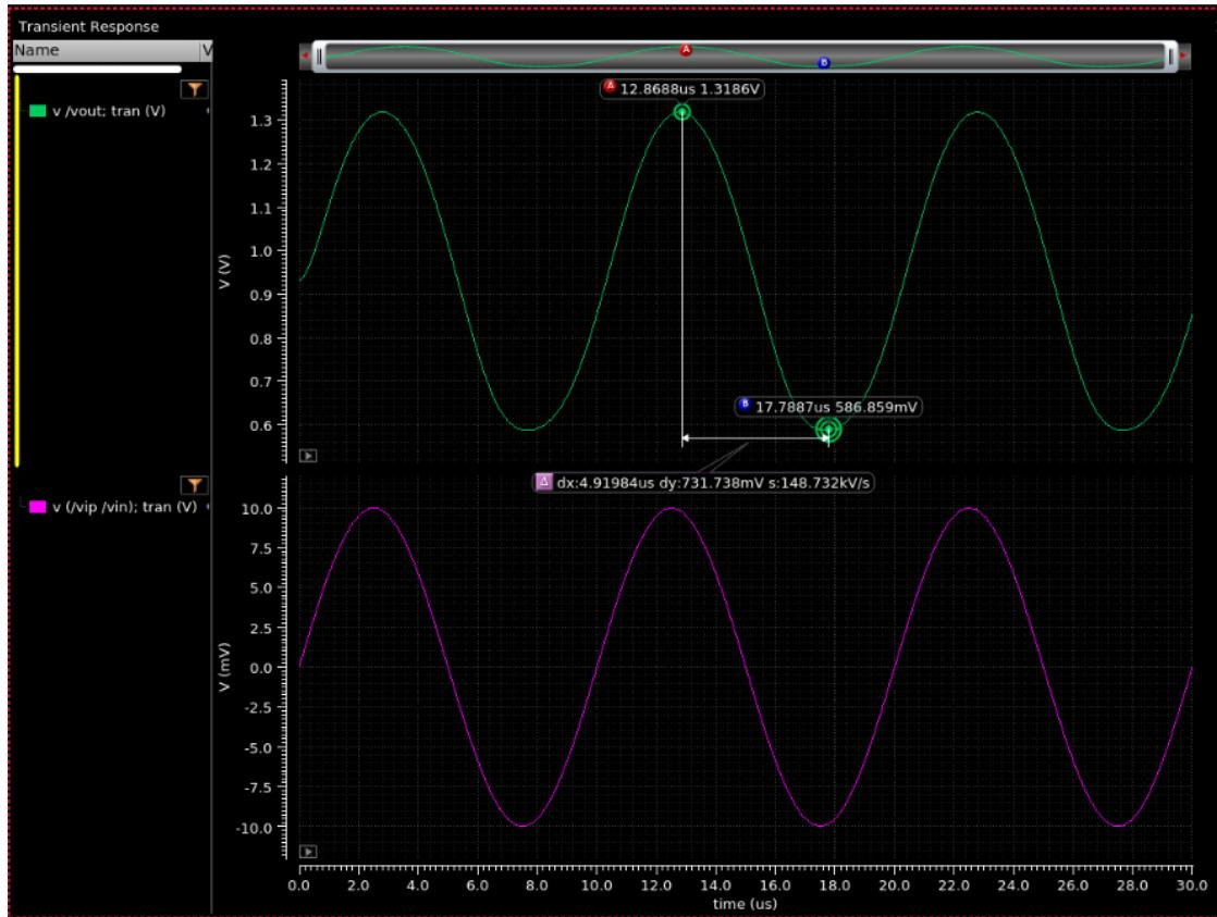
From the plot, we see that the differential input = 20mVpp, and the single-ended output is 732mVpp. This corresponds to a gain of 36.6V/V ( $20\log_{10}(36.6) = 31.2\text{dB}$ ). This matches well with the gain in the AC response.
