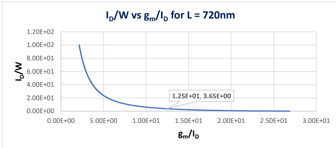
As can be seen from the plot, the value of  $I_D/W$  corresponding to  $g_m/I_D = 12.5$  is 3.65. Therefore,  $W_n = 20/3.65 = 5.5\mu\text{m} \approx 6\mu\text{m}$ . Yes, yes, we get what to do now. Fill the table!
