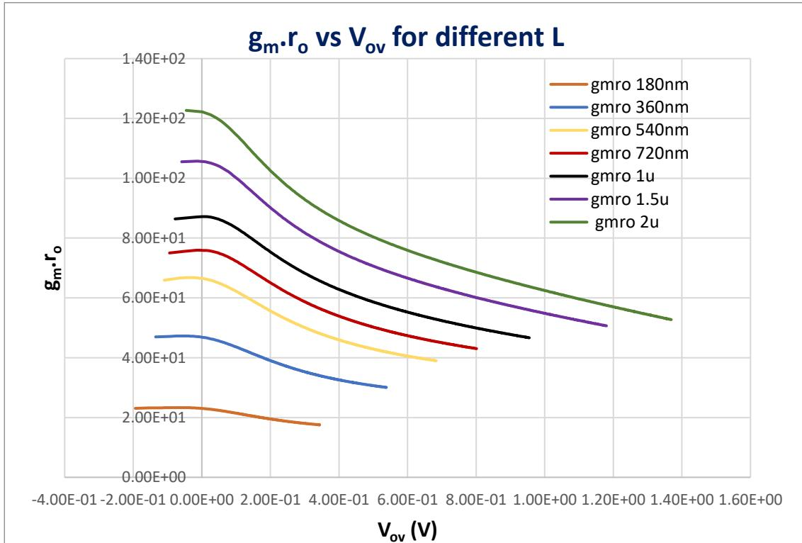
To identify the minimum length needed to meet the gain requirement in (1), we plot the  $g_m \cdot r_o$  as a function of  $V_{ov}$  for different values of  $L$ . From the plot, we notice that for  $L < 720\text{nm}$ , the gain specification cannot be satisfied. So, the minimum length required to meet the gain specification = 720nm. In our excitement, let us quickly fill the table 😊
