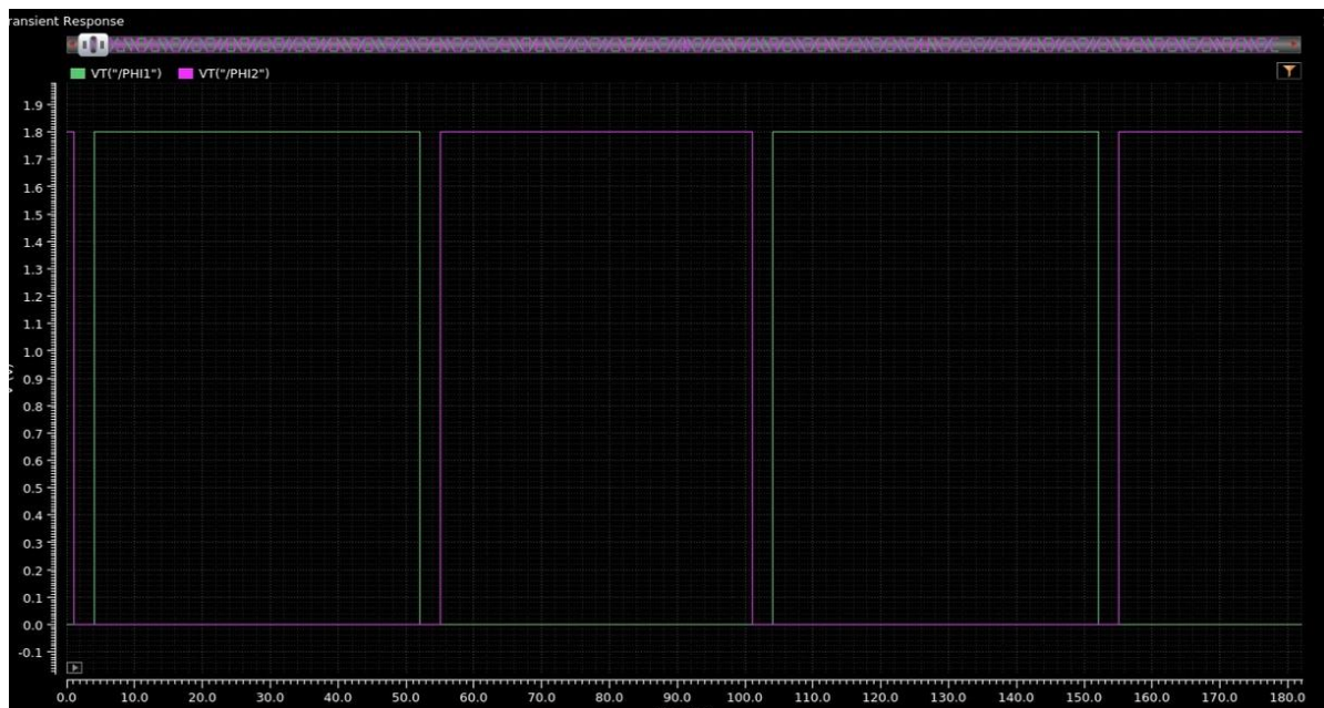
Fig. 4: Transient Simulation of Non-Overlapping Clock Generator
