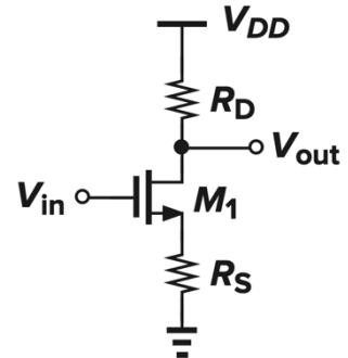
$$\overline{V_{n,out}^2} = 4kT R_D + 4kT \gamma \times \frac{1}{g_m} \times \left( \frac{g_m R_D}{g_m R_S + 1} \right)^2 + \frac{4kT}{R_S} \times \left( \frac{R_S}{R_S + \frac{1}{g_m}} \right)^2 \times R_D^2$$
