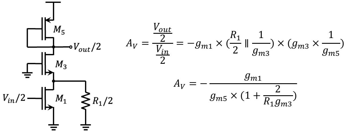
$$A_V = \frac{\frac{V_{out}}{2}}{\frac{V_{in}}{2}} = -g_{m1} \times \left( \frac{R_1}{2} \parallel \frac{1}{g_{m3}} \right) \times \left( g_{m3} \times \frac{1}{g_{m5}} \right)$$
