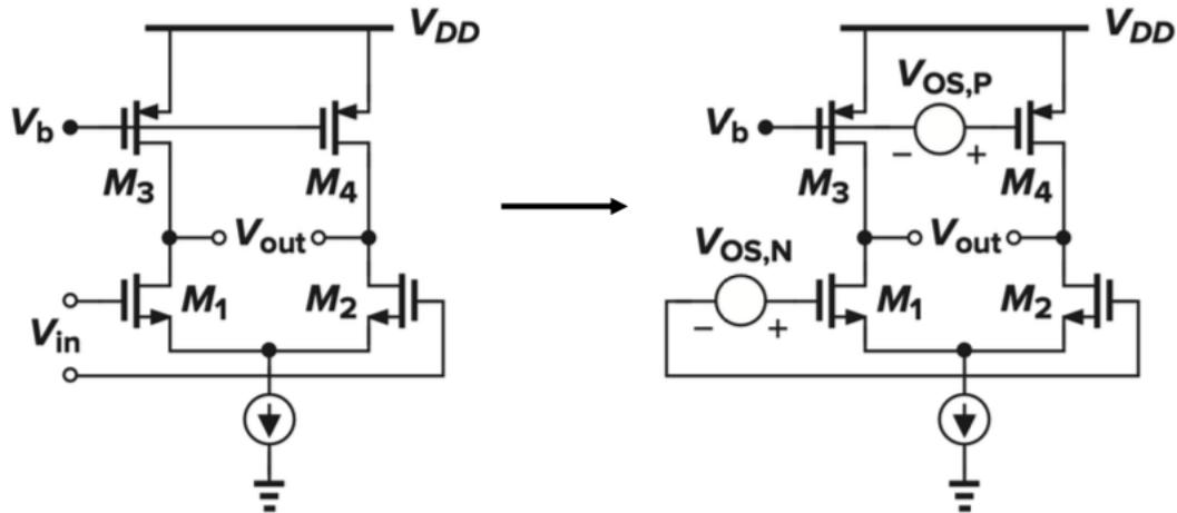
We insert the offsets of the NMOS and PMOS pairs.
