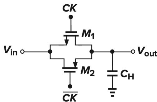
3. For the complementary switch shown below, find the condition for which the effect of charge injection by NMOS is canceled by that of PMOS.
