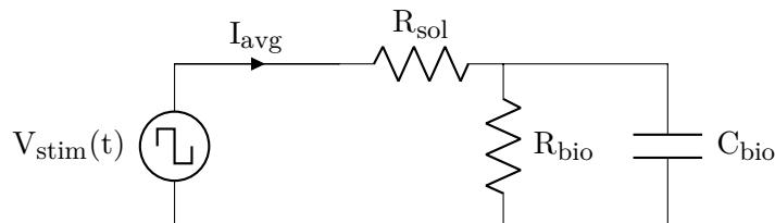
where the voltage step generator (period  $T$  and step voltage  $V_{\text{step}}$ ) polarizes the bio/nano layer modeled as a resistance  $R_{\text{bio}}$  and a capacitor  $C_{\text{bio}}$ . The voltage drop across the solution resistance is neglected so that the average current through the bio/nano layer is
