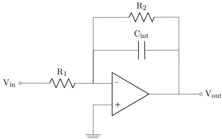
By applying nodal voltage analysis at the virtual ground of the opamp,
