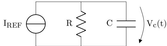
where  $R$  and  $C$  represent the contributions of resistive and capacitive elements variations at the electrode/solution interface. By applying Kirchhoff current law,
