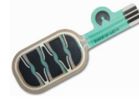
FSR: Force Sensing Resistor
