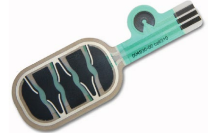
FSR: Force Sensing Resistor
