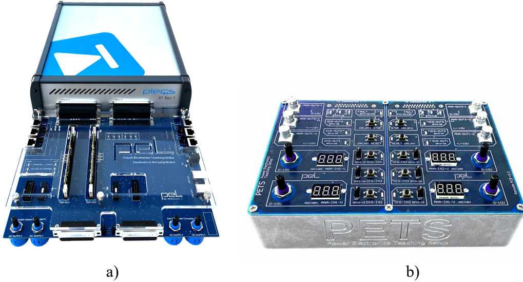
Fig. 5 a) The PETS HIL board developed to support control software development and testing, together with the RT Box creates the exact digital twin of the PETS. b) The PETS Remote board.
