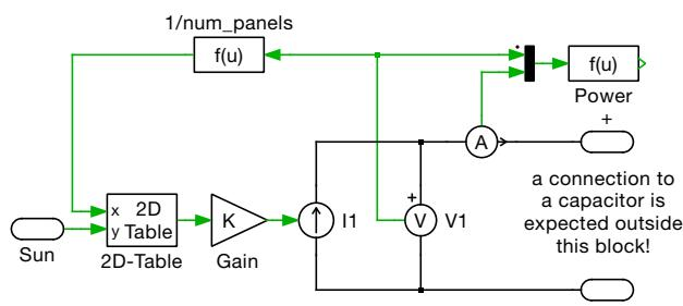
Fig. 1 PV panel model in PLECS.
