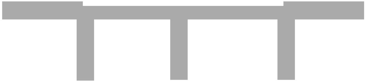
Fig. 7.15 : Microstrip line layout of a 3 stage low pass filter
