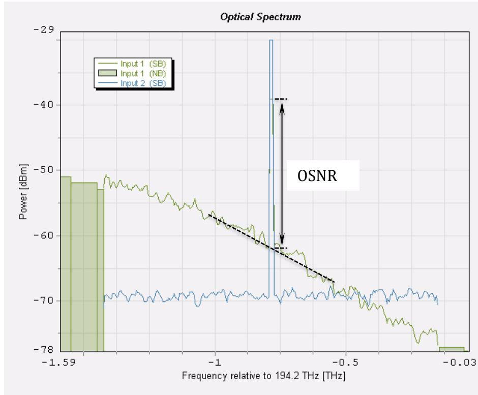
**Question 5:** Run *Sweep\_iterations* (the same simulation will be performed 11 times, and results are averaged out), and determine OSNR, gain and NF of the amplifier.
