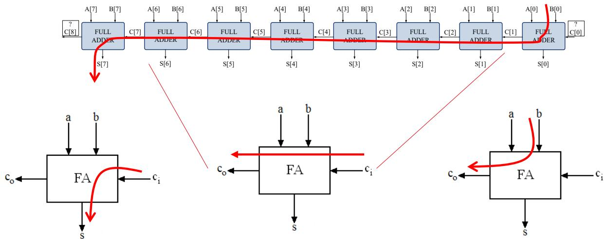
*Hint 1 : you may want to have different cells for the last, middle, and last adders of the chain. i.e., prune the un-necessary parts of the adder.*
