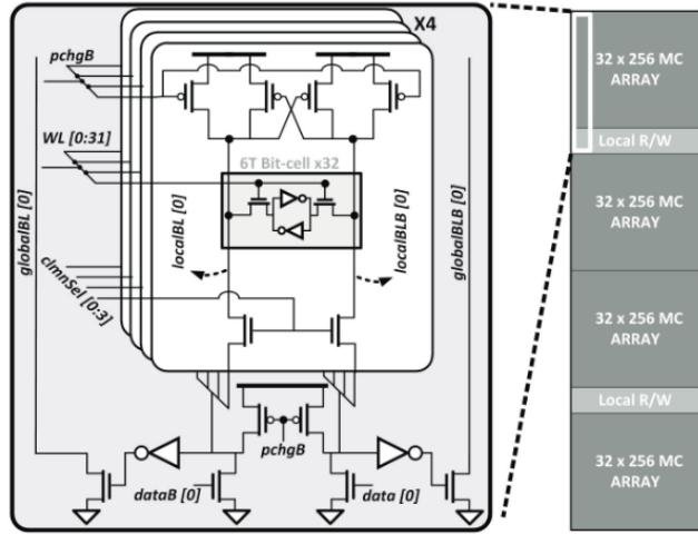
Each block composing a SRAM array has to be designed with the full custom flow as you did learn during phase 1 of these labs. As today memory compose more than 50% of the area of advanced chips, being able to automate the design of such blocks is mandatory.
