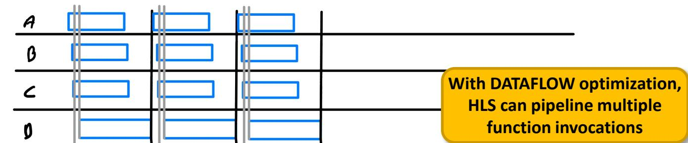
E.g., process 3 independent images, each one analyzed row-by-row. The functions can be pipelined by rows for each image
