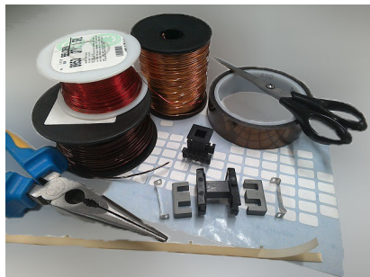
Figure 4 Tools and material available to set and trim the air gap length
