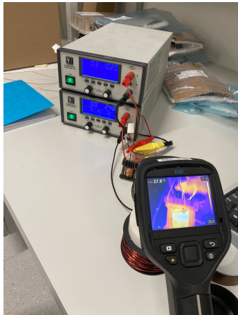
Figure 11 Heat-run test setup
