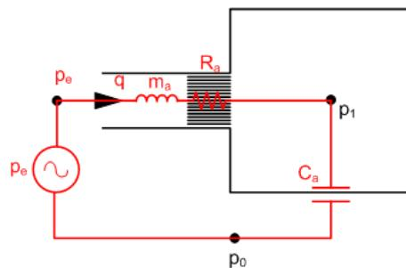
$$3. \frac{q}{p_e} = \frac{j\omega}{(j\omega)^2 m_a + j\omega R_a + \frac{1}{C_a}}.$$
