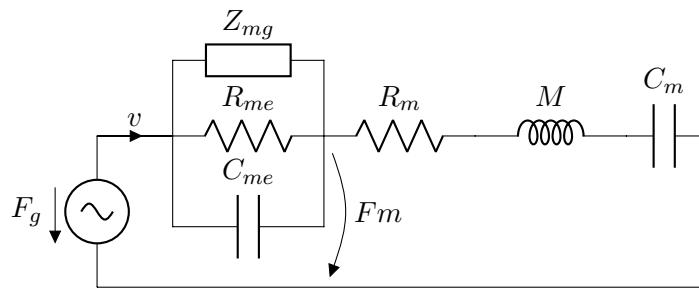
$$\begin{aligned} F_g &= u_g \frac{Bl}{Z_g + R_e + j\omega L_e} \\ Z_{mg} &= \frac{(Bl)^2}{Z_g} \\ R_{me} &= \frac{(Bl)^2}{R_e} \\ C_{me} &= \frac{L_e}{(Bl)^2} \end{aligned}$$
