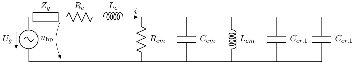
$$C_{er} = \frac{(Bl)^2}{S^2 M_{ar}} \quad L_{em} = (Bl)^2 C_m \quad R_{em} = \frac{(Bl)^2}{R_m} \quad C_{em} = \frac{M}{(Bl)^2}$$
