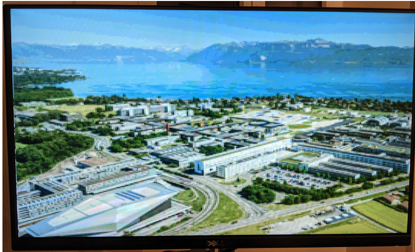
Figure 3: A successful implementation of a VGA controller with the described modification for the top-level should show an image of EPFL. In some cases there may be black borders depending on your screen size. The use of an HDMI adapter may also cause some flicker on the screen which is acceptable.
