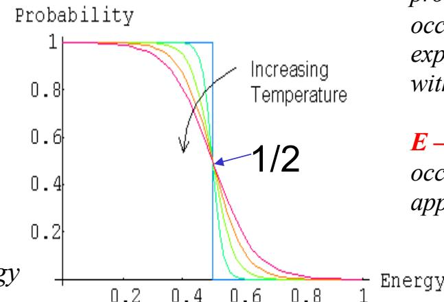
$E - E_F \gg kT$  - the probability of a state being occupied decreases exponentially with increasing  $E$
