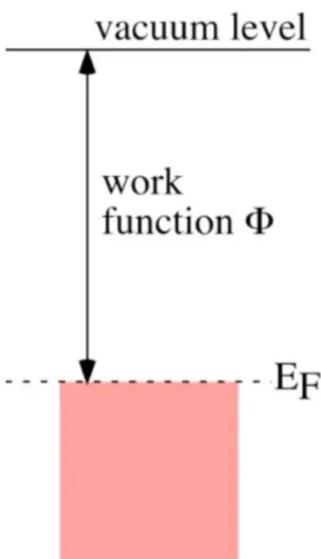
The work function  $\Phi$  refers to removal of an electron to a position that is far enough from the surface (many nm) that the force between the electron and its image charge in the surface can be neglected (vacuum level)
