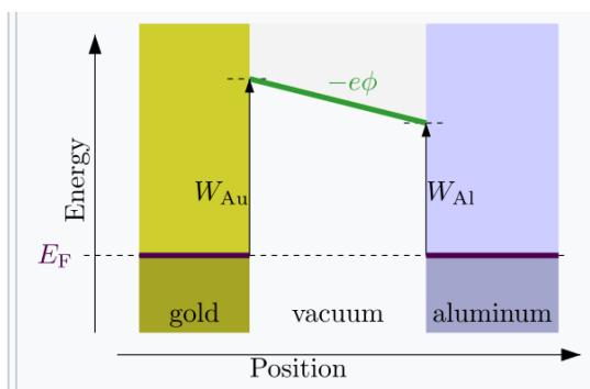
Here is a system with two different metals (Au and Al), with work functions of 5.5eV and 4.1eV
