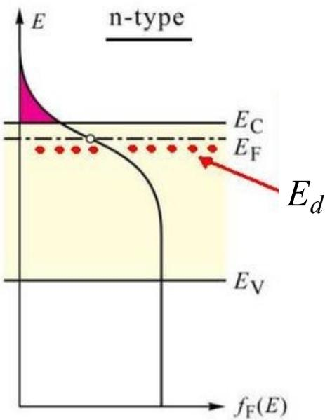
For donors, the difference ( $E_d - E_F$ ) determines the degree of ionization
