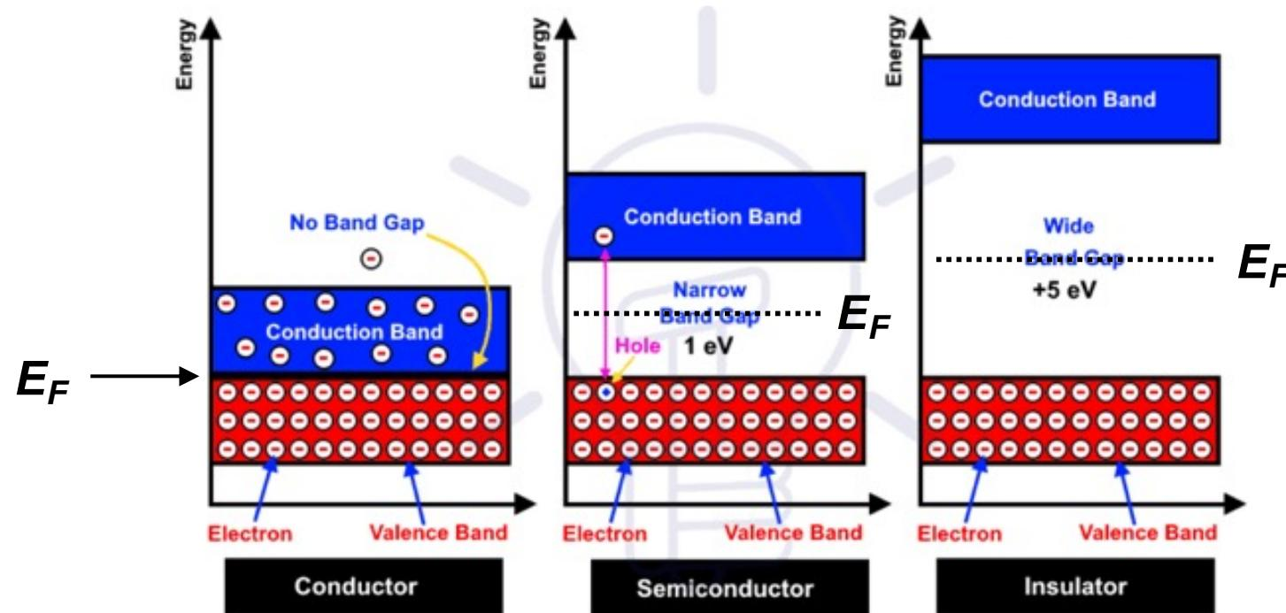
In semiconductors and insulators the Fermi level is situated within the band gap (forbidden band)
