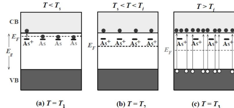
(a) Below  $T_s$ , the electron concentration is controlled by the ionization of the donors. (b) Between  $T_s$  and  $T_i$ , the electron concentration is equal to the concentration of donors since they would all have ionized. (c) At high temperatures, thermally generated electrons from the VB exceed the number of electrons from ionized donors and the semiconductor behaves as if intrinsic.
