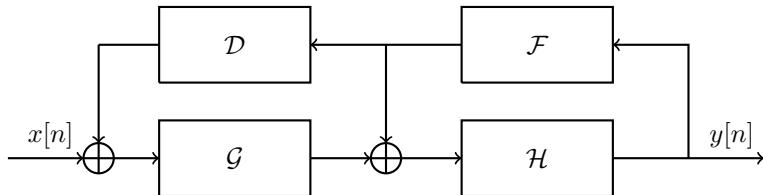
What is the overall transfer function of the system as a function of  $D(z)$ ,  $F(z)$ ,  $G(z)$  and  $H(z)$ ?
