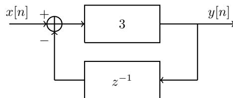
where recall that the labels 3 and  $z^{-1}$  denote the transfer functions for the two composed systems
