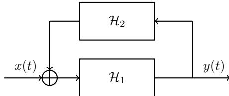
(a) Suppose  $H_1(s) = 1$  and  $H_2(s) = \frac{1}{s}$ , what is the transfer function  $H(s)$  of the overall system  $\mathcal{H}$ ? The overall system  $\mathcal{H}$  is known to be causal, is it also stable? Find its impulse response  $h(t)$ .
