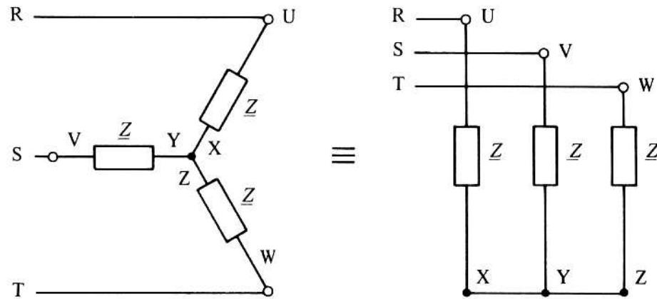
$$I_{UX} = \frac{\underline{U}_{UX}}{\underline{Z}} = \frac{\underline{U}_{RN}}{\underline{Z}} = \frac{\underline{U}}{\underline{Z}} e^{j(\alpha - \varphi)}$$
