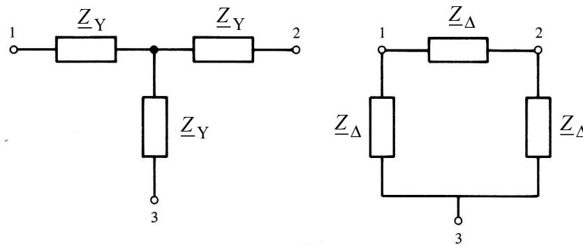
$$\underline{Z}_Y = \frac{\underline{Z}_\Delta}{3} \quad \leftrightarrow \quad \underline{Z}_\Delta = 3\underline{Z}_Y$$
