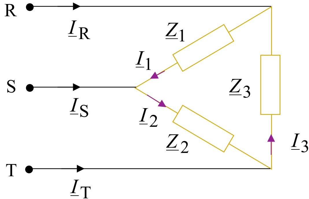
$$\underline{I}_R = \underline{I}_1 - \underline{I}_3 = 224.1 - j147.4 \text{ A} = 268.2 e^{-j33.3^\circ} \text{ A}$$
