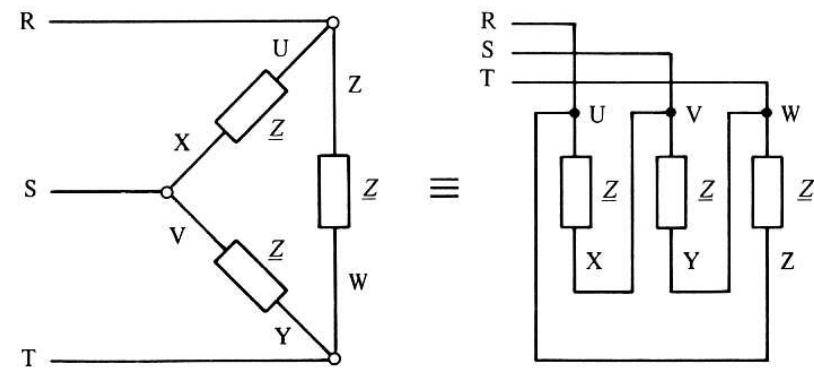
$$I_{UX} = \frac{\underline{U}_{UX}}{\underline{Z}} = \frac{\underline{U}_{RS}}{\underline{Z}} = \frac{\sqrt{3}U}{Z} e^{j(\alpha - \varphi + \pi/6)}$$
