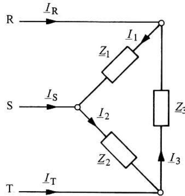
$$\underline{I}_R = \underline{I}_1 - \underline{I}_3 \quad \underline{I}_S = \underline{I}_2 - \underline{I}_1 \quad \underline{I}_T = \underline{I}_3 - \underline{I}_2$$
