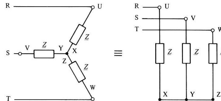
$$\underline{I}_R = \underline{I}_{UX} \quad \underline{I}_S = \underline{I}_{VY} \quad \underline{I}_T = \underline{I}_{WZ}$$
