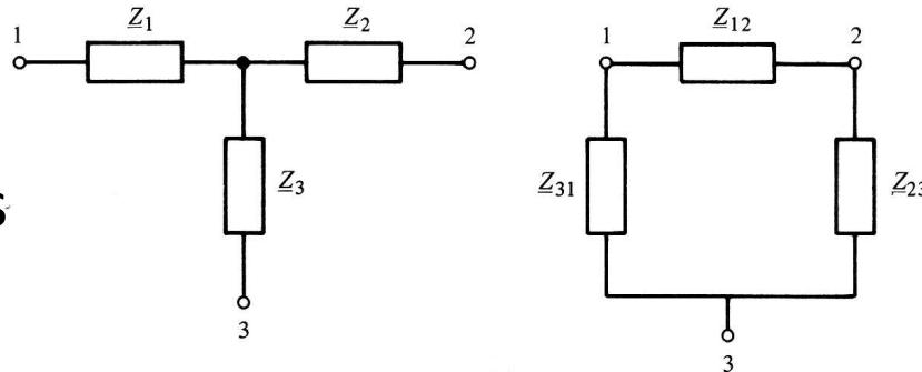
$$\underline{Z}_{12} = \frac{\underline{Z}_1 \underline{Z}_2 + \underline{Z}_2 \underline{Z}_3 + \underline{Z}_3 \underline{Z}_1}{\underline{Z}_3}$$
