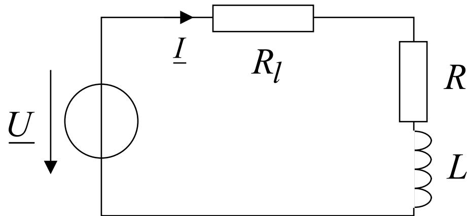
Pertes dans la ligne:  $P_l = R_l I^2 = R_l I \frac{U}{\sqrt{R^2 + (\omega L)^2}} = \frac{R_l U I \sin \varphi}{\omega L}$
