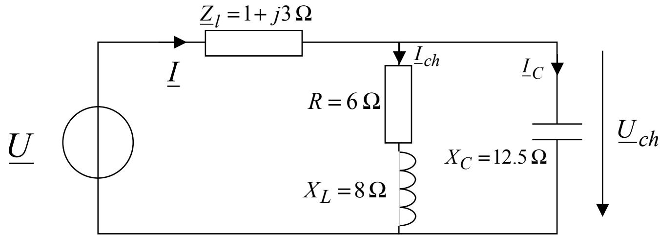
$$\underline{I}_C = \frac{\underline{U}_{ch}}{Z_C} = \frac{250}{12.5e^{-j90^\circ}} = 20e^{j90^\circ} \text{ A}$$
