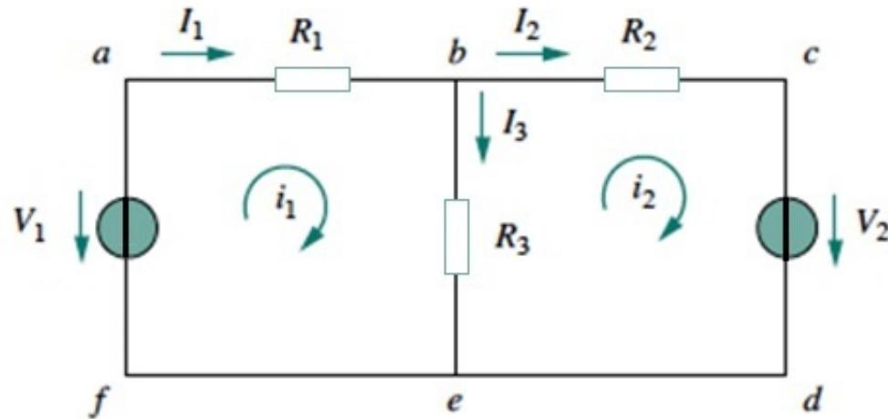
$$\text{Maille 1: } -V_1 + R_1 i_1 + R_3 (i_1 - i_2) = 0 \quad \text{ou:} \quad (R_1 + R_3) i_1 - R_3 i_2 = V_1$$
