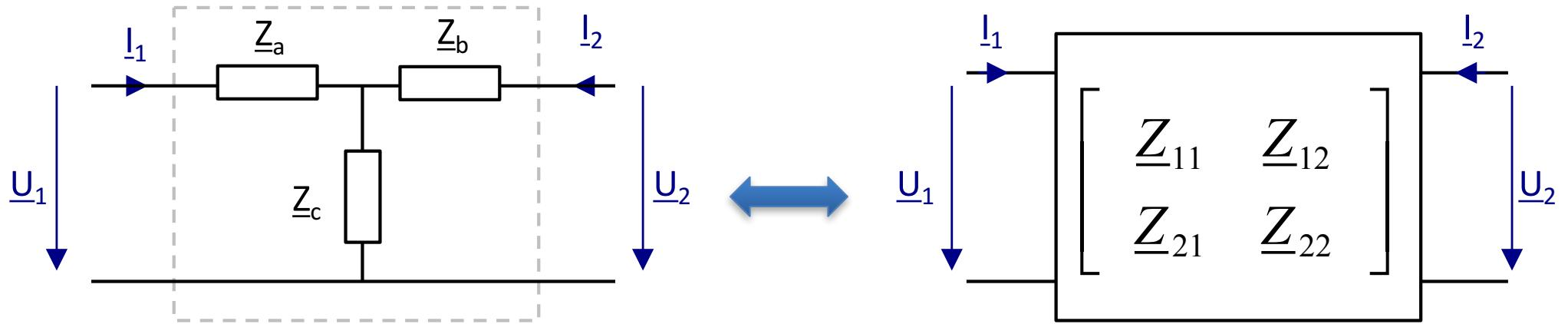
$$\underline{Z}_{11} = (\underline{Z}_a + \underline{Z}_c); \quad \underline{Z}_{22} = (\underline{Z}_b + \underline{Z}_c); \quad \underline{Z}_{12} = \underline{Z}_{21} = \underline{Z}_c$$
