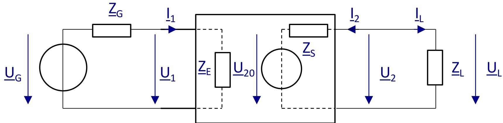
$$\underline{Z}_E = \frac{\underline{U}_1}{\underline{I}_1} = \underline{Z}_{11} - \frac{\underline{Z}_{12}\underline{Z}_{21}}{\underline{Z}_{22} + \underline{Z}_L}$$
