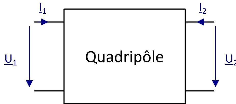
$$\begin{bmatrix} \underline{U}_1 \\ \underline{U}_2 \end{bmatrix} = \begin{bmatrix} \underline{Z}_{11} & \underline{Z}_{12} \\ \underline{Z}_{21} & \underline{Z}_{22} \end{bmatrix} \begin{bmatrix} \underline{I}_1 \\ \underline{I}_2 \end{bmatrix} \Leftrightarrow \begin{cases} \underline{U}_1 = \underline{Z}_{11}\underline{I}_1 + \underline{Z}_{12}\underline{I}_2 \\ \underline{U}_2 = \underline{Z}_{21}\underline{I}_1 + \underline{Z}_{22}\underline{I}_2 \end{cases}$$
