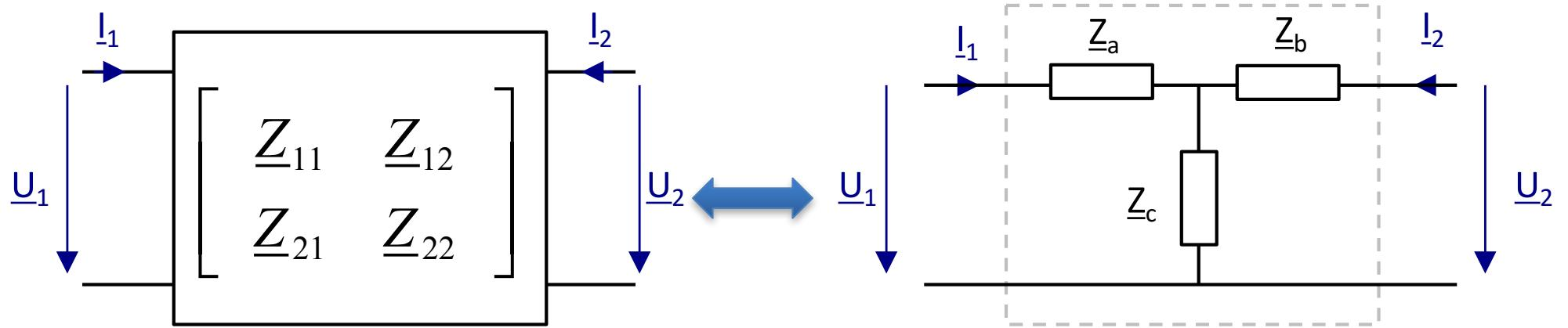
$$\underline{Z}_a = (\underline{Z}_{11} - \underline{Z}_{12}); \quad \underline{Z}_b = (\underline{Z}_{22} - \underline{Z}_{12}); \quad \underline{Z}_c = \underline{Z}_{12}$$
