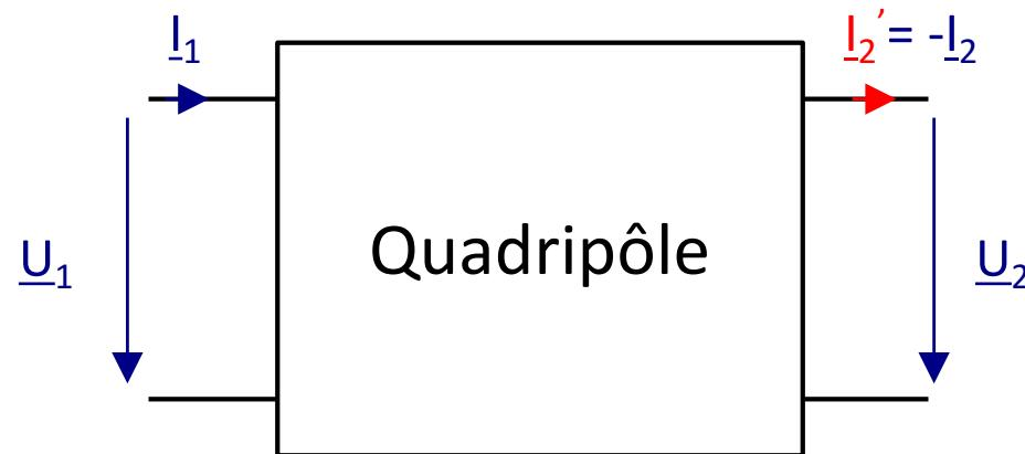
$$\begin{bmatrix} \underline{U}_1 \\ \underline{I}_1 \end{bmatrix} = \begin{bmatrix} \underline{A} & \underline{B} \\ \underline{C} & \underline{D} \end{bmatrix} \begin{bmatrix} \underline{U}_2 \\ -\underline{I}_2 \end{bmatrix} \Leftrightarrow \begin{cases} \underline{U}_1 = \underline{A}\underline{U}_2 - \underline{B}\underline{I}_2 \\ \underline{I}_1 = \underline{C}\underline{U}_2 - \underline{D}\underline{I}_2 \end{cases}$$
