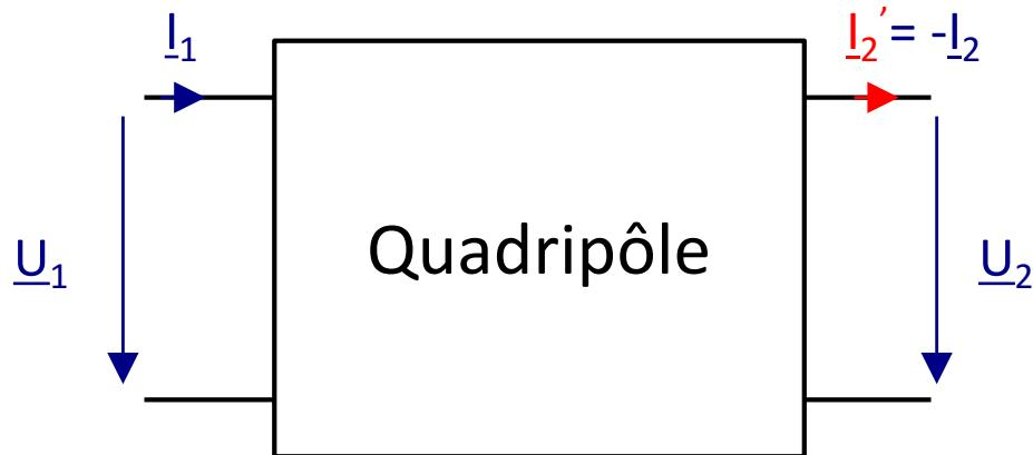
$$\begin{bmatrix} \underline{U}_2 \\ -\underline{I}_2 \end{bmatrix} = \begin{bmatrix} \underline{D} & -\underline{B} \\ -\underline{C} & \underline{A} \end{bmatrix} \begin{bmatrix} \underline{U}_1 \\ \underline{I}_1 \end{bmatrix}$$
